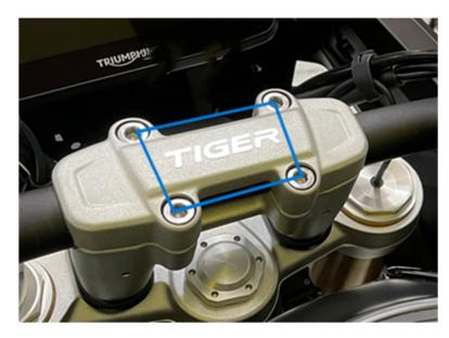
Handlebar positioned to the front of the upper triple clamp.
