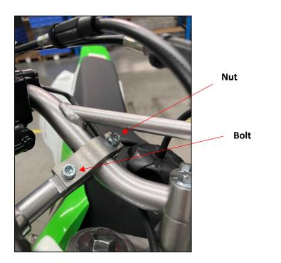
• Clutch and brake levers may need to be moved towards the centre slightly to allow clearance between the ends of the levers, and the side of the backbone.
