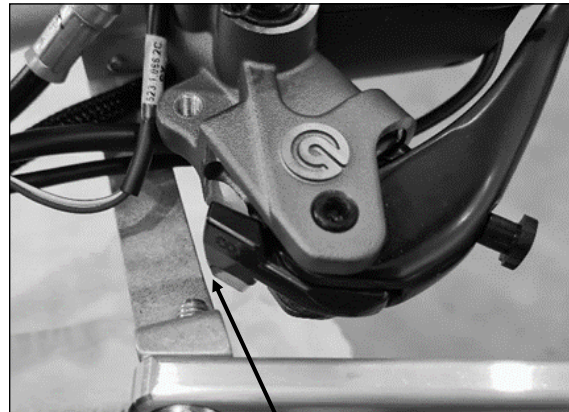
Pull clutch in all the way and ENSURE there is at least 2-3mm clearance between the mounting bracket and inner end of clutch lever
