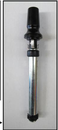
**TIPS:** To help with applying lubrication to the inside of the handlebar, loosen throttle housing and slide inwards. For left side use a screwdriver to lever grip end away from handlebar end. Be careful not to get lubrication between grip and outside of handlebar.
