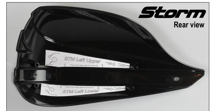
**NOTE:** Photos indicate correct placement of Drilling Templates on **REAR** of guard. Secure with clear tape prior to drilling.
